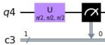
Figure 2: A circuit where the quantum bit is rotated and then measured. The measurement result is stored in a classical register.
